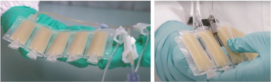
Figure 2. Filling and sealing multi-chamber (b) (4) bags
